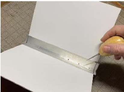
holes are punched with an awl through the 4 pages of each signature using a spacing template
