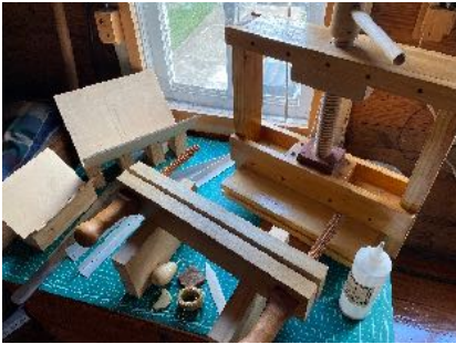
basic bookbinding tools, including cradles for punching sewing holes, a book press and a finishing or laying in press all made here in the shop
