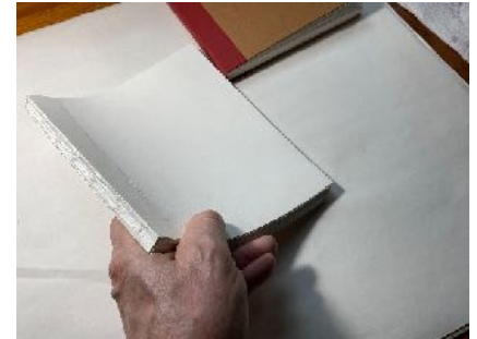
the finished book block with signatures sewn and glued on the spine, end pages attached and a narrow wrapper added for strengthening
